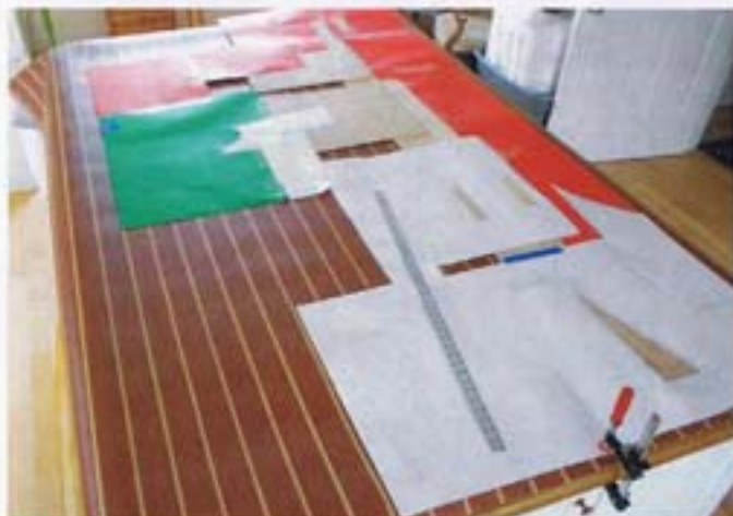
As the Lonseal material came in a large sheet, Art made a one-piece template for the saloon sole, at top, by taping poster board to a backbone of thin plywood. He laid the template on the material, at left, and used tape to transfer the shape and create a line to cut to. Roughed in, at right, the new sole fits nicely.
