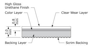
Note: M668UV differs with no clear wear layer, a thicker backing layer, and a total wear layer thickness of 0.45 mm.
